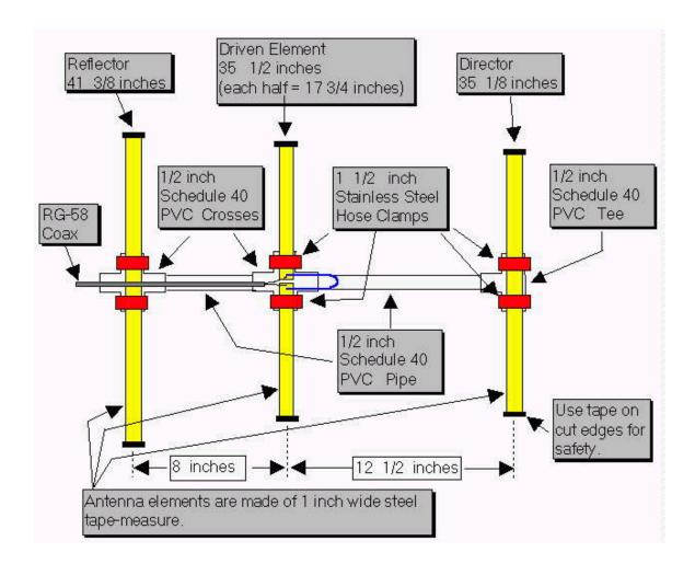
I used 1 1/2 inch hose clamps to attach all the elements on my prototype beam. Others who have duplicated my design have used self-tapping screws to attach the elements to the PVC crosses and Tees. Performance is the same using either method. The screws are much less expensive but they do not hold the elements as securely. If you do not use 1/2 inch PVC fittings but instead use 3/4 inch, make sure the hose clamps you buy are large enough to fit.
